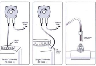
When inserting chlorine and acid tubes into dosing cell, tubes should penetrate approximately 50mm or half way into the depth of the mixing chamber. If the tube has a radius formed which is caused by the memory of the material, it is important that the tube point in the direction of the water flow.
